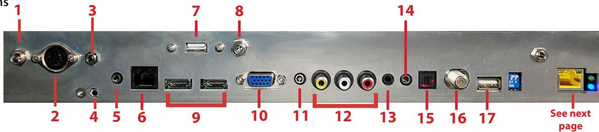
1. **2.5mm power jack** - 12v @ 3amps Auxillary power supply
