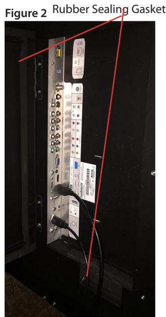
Route cables trough the bottom of the door only
